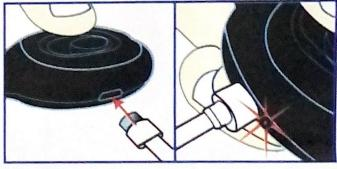
Plug USB end of cable into a power adapter or computer, then insert micro-USB tip into the charging port on side.
