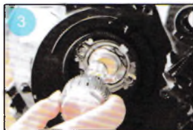
Accurated the LED lamp alignment buttons for installation.
